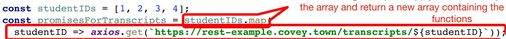
Functional magic: map will apply the function specified to each element in the array and return a new array containing the result of each of those
