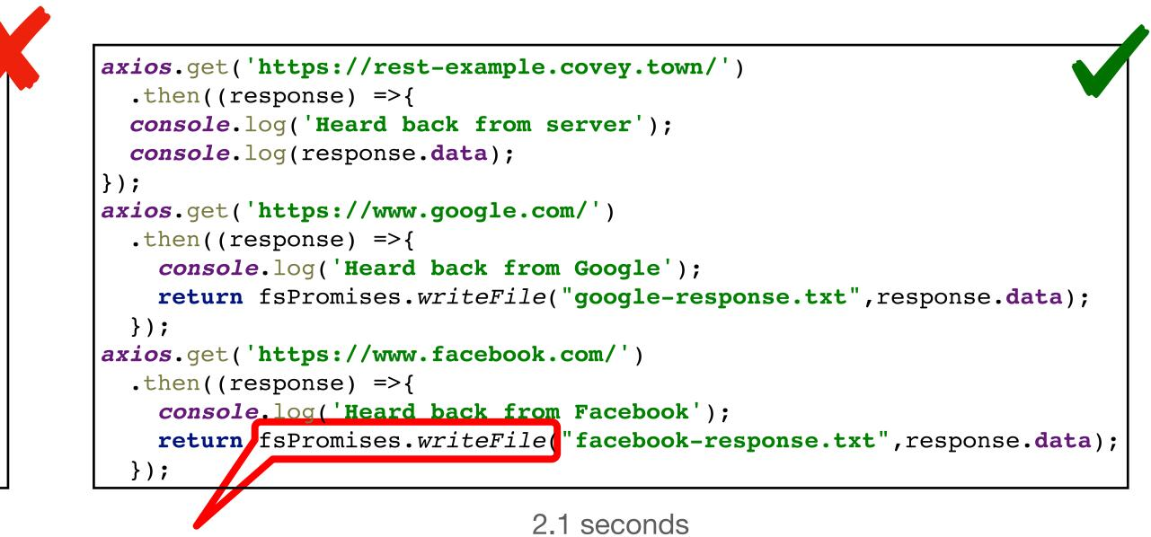
Write a file asynchronously (Ask NodeJS to write it in the background, this returns a new Promise to tell us when it's done)
